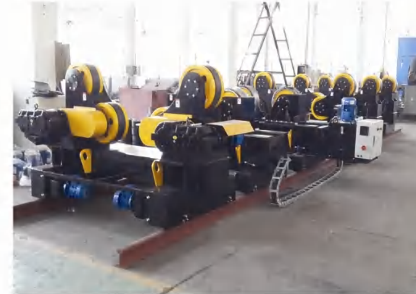
60T 电动行走滚轮架配组对 60Ton Motorized Moving Welding Rotator with Fit-Up (Midland,TX)
