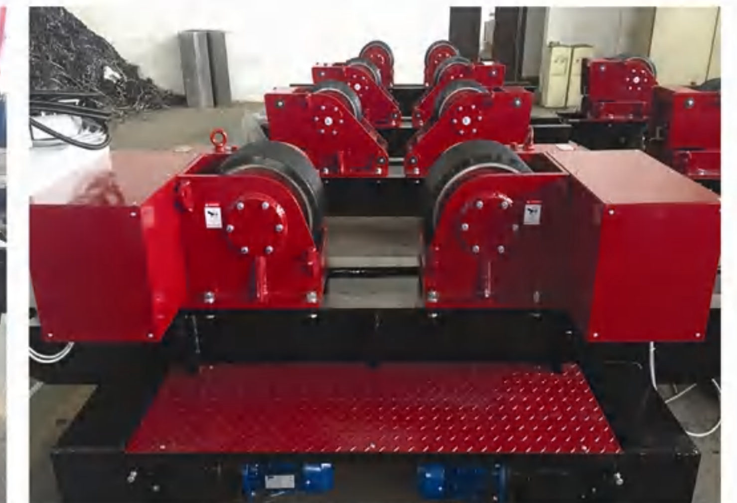
40Ton 标准组对中心 (10Ton-500Ton) 40Ton Standard Fit-up Growing Line (Brisbane, Australia)
