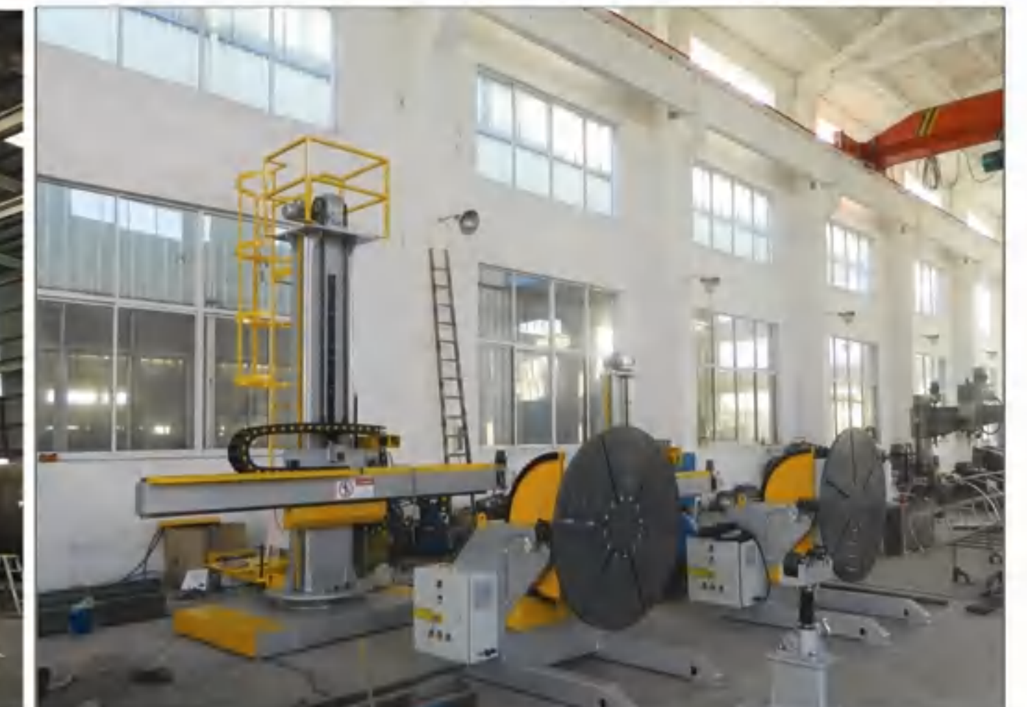
小型操作机配变位机 1.5x1.5 Small Welding Manipulator with Welding Positioner (Toronto, Canada)
