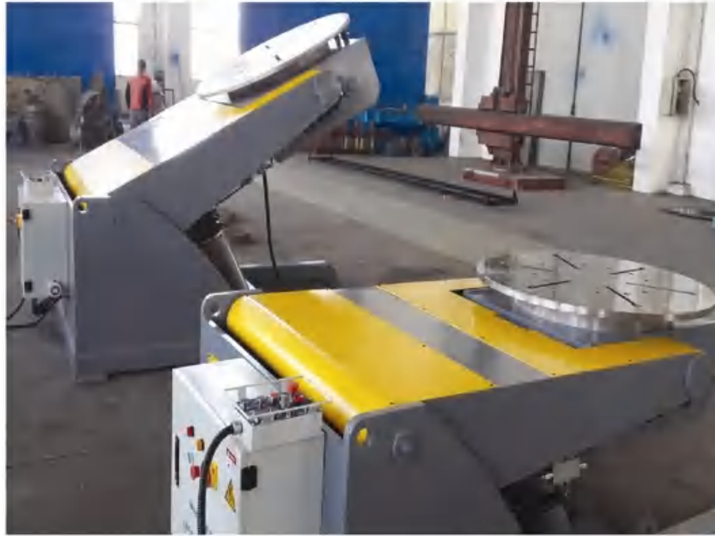
3Ton & 5Ton 3轴液压焊接变位机 3Ton & 5Ton 3Axis Hydraulic Welding Positioner (Dubai, UAE)
