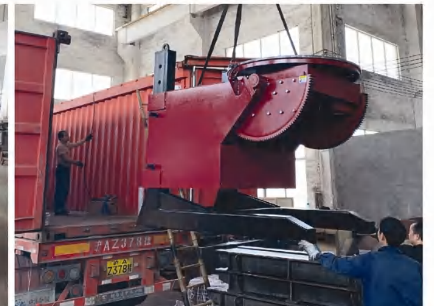
5Ton 手动升降焊接变位机装箱 Loading of 5Ton Manual Elevating Welding Positioner
