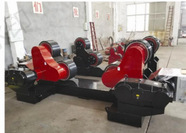
150Ton 双驱聚氨酯自调滚轮架 150Ton Polyurethane Wheel Welding Rotator (Rayong,Thailand)
