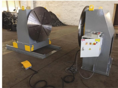
3Ton 特制头尾式焊接变位机 3Ton Customized Head Tail Stock Welding Positioner (Singapore)
