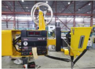
林肯NA-5控制器配送丝机, 机头 (埋弧焊) Lincoln NA-5 Controller with Wire Feeder & Welding Torch (SAW)
