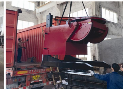
5Ton 手动升降焊接变位机装箱 Loading of 5Ton Manual Elevating Welding Positioner
