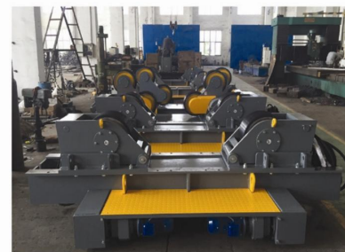
100Ton 特制组对中心 100Ton Customized Fit-up Welding Station (Vung tau, Vietnam)
