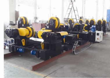
60T电动机行走滚轮架配组对 60Ton Motorized Moving Welding Rotator with Fit-Up (Midland,TX)
