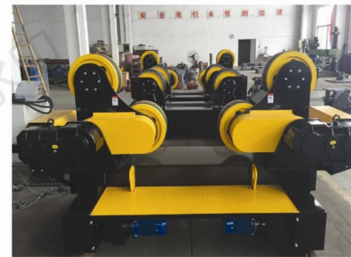
60Ton 自调滚轮架配平移式组对滚轮架 60Ton Self-aligning rotator with Translational type fit-up (Midland, TX)
