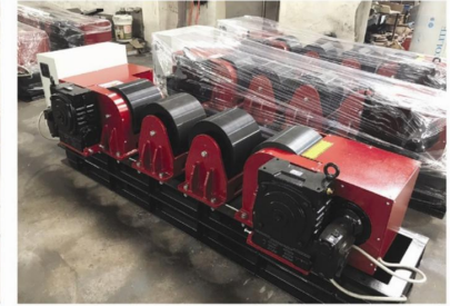
30Ton 聚氨酯轮特制可调滚轮架 30Ton PU Wheel Welding Rotator (Brisbane, Australia)
