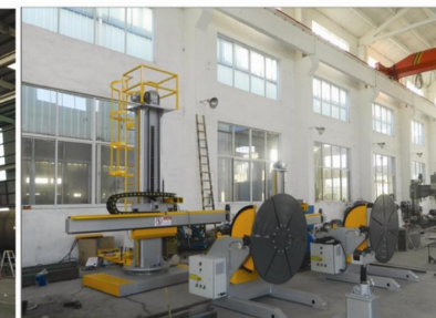
小型操作机配变位机 1.5x1.5 Small Welding Manipulator with Welding Positioner (Toronto, Canada)
